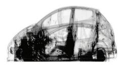
Above is a representative image of a car scanned with a vehicle scanner that has its X-ray beams shooting from the side.
